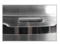
4. Safety Window - Fourth Safe Guard Safety window on the rim of the cover releases pressure in the pressure cooker if the other safety valves fail. The silicone gasket itself will push through the safety window to release pressure to ensure perfectly safe cooking, while the cover will stay on the pressure cooker without rupturing.
